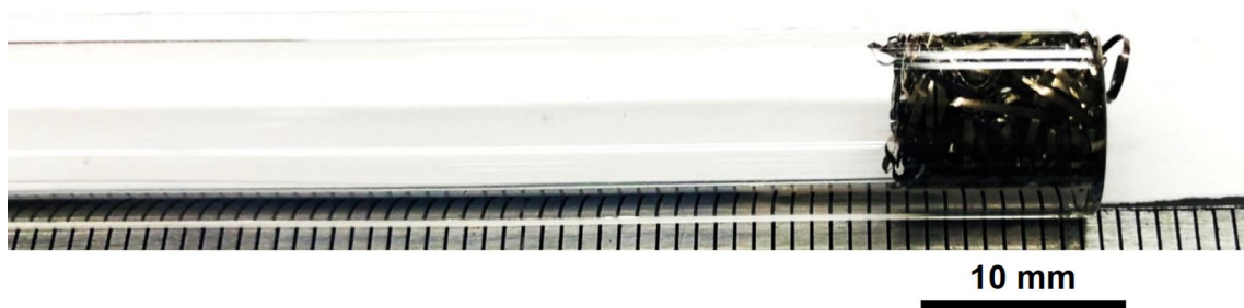
Fig. 38 OM image of Scrubber Cleanz pressed down toward the end of the stem tube
