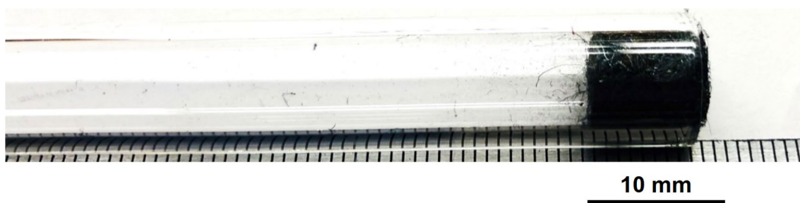
Fig. 40 OM image of Rhodes American steel wool as-pressed to end of tube
