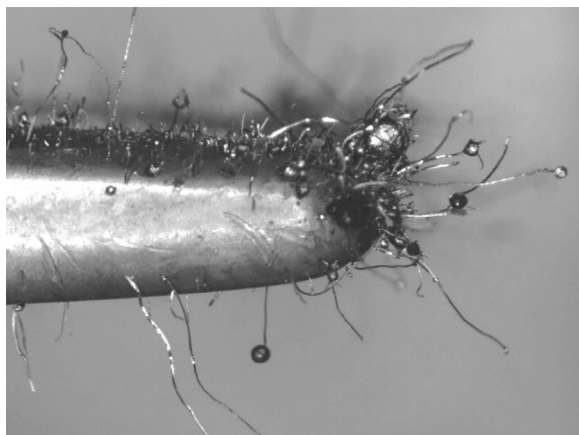
Fig. 68 As-heated Rhodes American fragments recovered from the tube interior by the tip of magnetized tweezers
