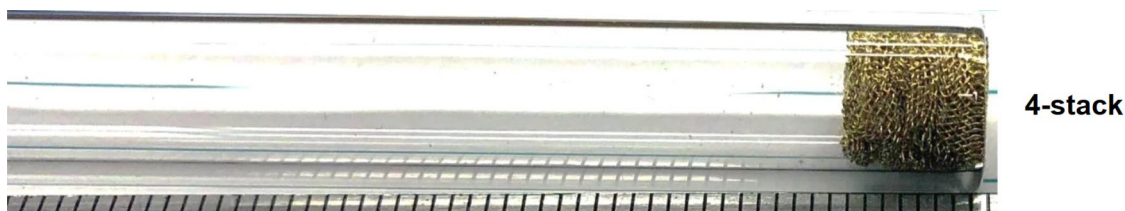
Fig. 34 OM image of four Impact 1.0 screens stacked and pressed down the stem tube
