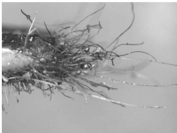
Fig. 69 As-heated S.O.S. fragments recovered from the tube interior by the tip of magnetized tweezers
