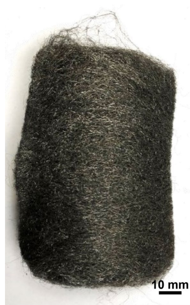
Fig. 25 OM image of as-received Rhodes American steel wool
