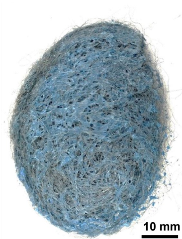
Fig. 29 OM image of as-received S.O.S. steel wool pad
